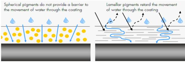
(Steel is chemically unstable - it rapidly rusts in the presence of oxygen and moisture to form iron oxide (rust). Iron oxide is however chemically stable as it cannot rust any further. Iron oxide is therefore an excellent pigment, and MIO is even better when it comes to the protection of steel).
